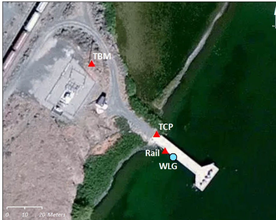
Figure 4. Water level gauge (WLG), RAIL point, temporary control point (TCP) and USACE temporary benchmark (TBM).
